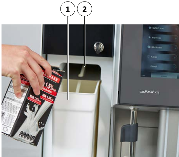
Fig. 11: Filling the milk container
