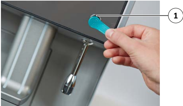
Fig. 3: Logging in with a chip key
