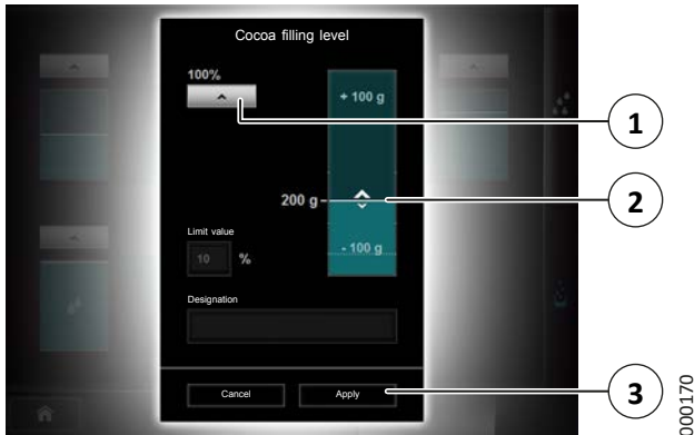
Fig. 13: Adjusting filling levels more accurately
