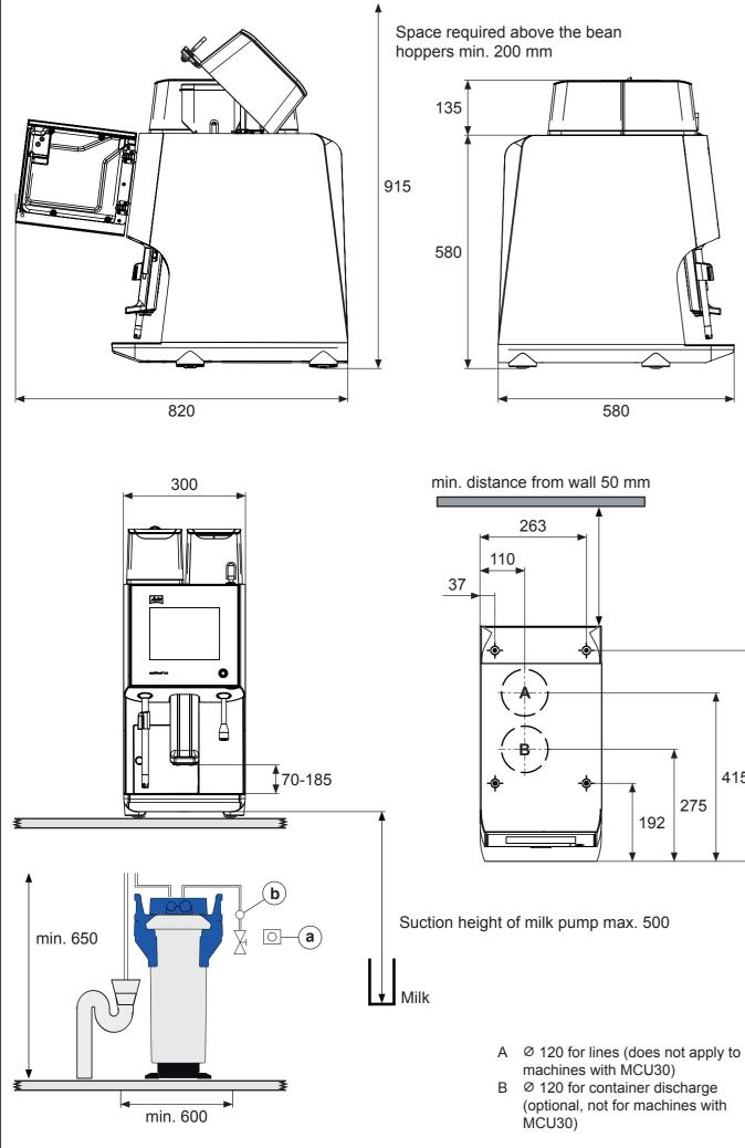
The Melitta<sup>®</sup> Cafina<sup>®</sup> XT5 is delivered ready for connection. However, before setting it up, the connections required on site must have been installed within a radius of 1 m so that they are easily accessible. This preliminary work must be carried out by authorized specialists in compliance with the applicable regulations. Melitta® Customer Service is not authorized to carry out this work and does not assume any responsibility for the installation.
