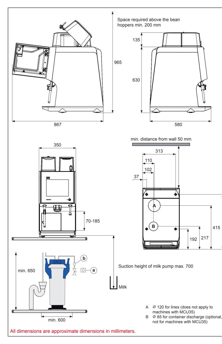
The Melitta<sup>®</sup> Cafina<sup>®</sup> XT8 is delivered ready for connection. However, before setting it up, the connections required on site must have been installed within a radius of 1 m so that they are easily accessible. This preliminary work must be carried out by authorized specialists in compliance with the applicable regulations. Melitta® Customer Service is not authorized to carry out this work and does not assume any responsibility for the installation.
