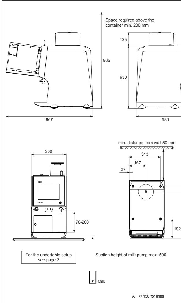
The Melitta® Cafina® XT8-F is delivered ready for connection. However, before setting it up, the connections required on site must have been installed within a radius of 1 m so that they are easily accessible. This preliminary work must be carried out by authorized specialists in compliance with the applicable regulations. Melitta<sup>®</sup> Customer Service is not authorized to carry out this work and does not assume any responsibility for the installation.
