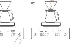
Put ground coffee with desired weight into the filter. Quick press the Tare button again.
