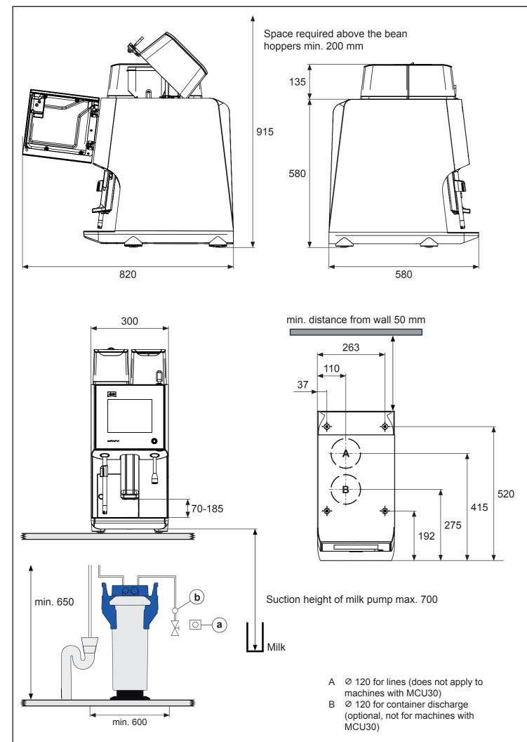
The Melitta® Cafina® XT7 is delivered ready for connection. However, before setting it up, the connections required on site must have been installed within a radius of 1 m so that they are easily accessible. This preliminary work must be carried out by authorized specialists in compliance with the applicable regulations. Melitta® Customer Service is not authorized to carry out this work and does not assume any responsibility for the installation.
