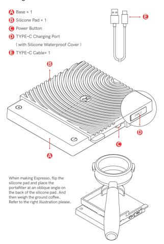
The base is a minimal-design panel with two touch keys.
