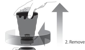
Remove the bean hopper from the motor base, push down and turn counterclockwise.
