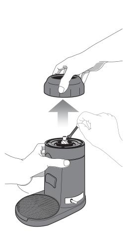
Lift the grind adjustment collar away from the motor base and clean with the brush. Clean the bottom burr using the burr cleaning brush.
