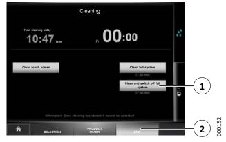
Fig. 5: Switching off the machine
