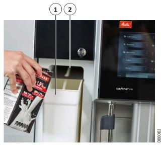
Fig. 10: Filling the milk container
