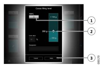
Fig. 12: Adjusting filling levels more accurately
