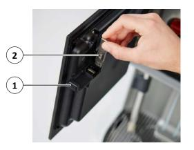
Fig. 36: Inserting the USB stick
