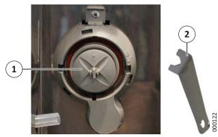
Fig. 44: Removing the mixer impeller
