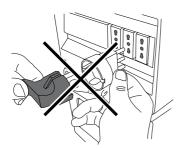
Make sure that the power cord plug is easily reachable after installation.
