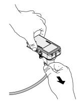
Remove the chrome-plated cover from the Cappuccinatore. Remove the valve from the Cappuccinatore.
