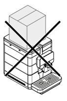
Due to the total weight, do not stack more than three machines on top of each other. The machine should be stored in its original packaging, in a dry and/or dust-FREE place. 5
