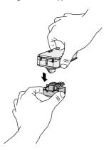
Turn and lift the Cappuccinatore cover and remove it from the Cappuccinatore body.
