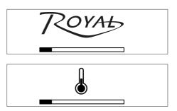
The progress bar indicates that the machine is heating up the system.
