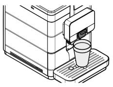
Press the "Coffee" button to start brewing. The machine starts brewing coffee from the dispensing spout. Wait until brewing has been completed and empty the container. Repeat the brewing process 3 times.
