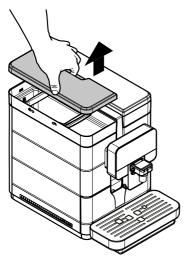
Remove the tank; lift it using the inside handles.
