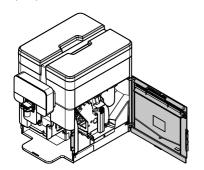
Close the door again and brew 1-2 cups of coffee to verify the changes in the grinding degree. Repeat the procedure until you reach the desired grind setting.
