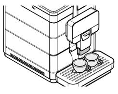
Push the dispensing spout towards the machine interior to its limit stop, to allow the use of tall glasses or MUGS. In this case, you can just brew one product at a time.
