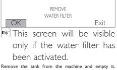
Remove the tank from the machine and empty it. Remove the anti-scale filter. Select "OK" and press the "OK" button. The following screen is displayed:
