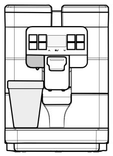
Press the "Hot Water" dispensing button. After a few moments hot water will be dispensed from the hot water dispensing spout.
