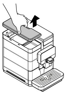
Remove the tank; lift it using the inside handles.
