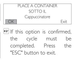
Place an empty container of at least I litre capacity under the dispensing spout and press the "OK" button to confirm. The machine performs a Cappuccinatore standard clean cycle.
