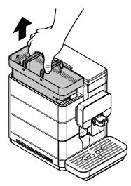
Rinse and fill it with fresh water; do not exceed the level (MAX) indicated on the tank.
