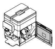
Remove the brew group by pulling it by the handle and pressing the «PRESS» button. The brew group must be washed with lukewarm water only. Do not use any detergent.
