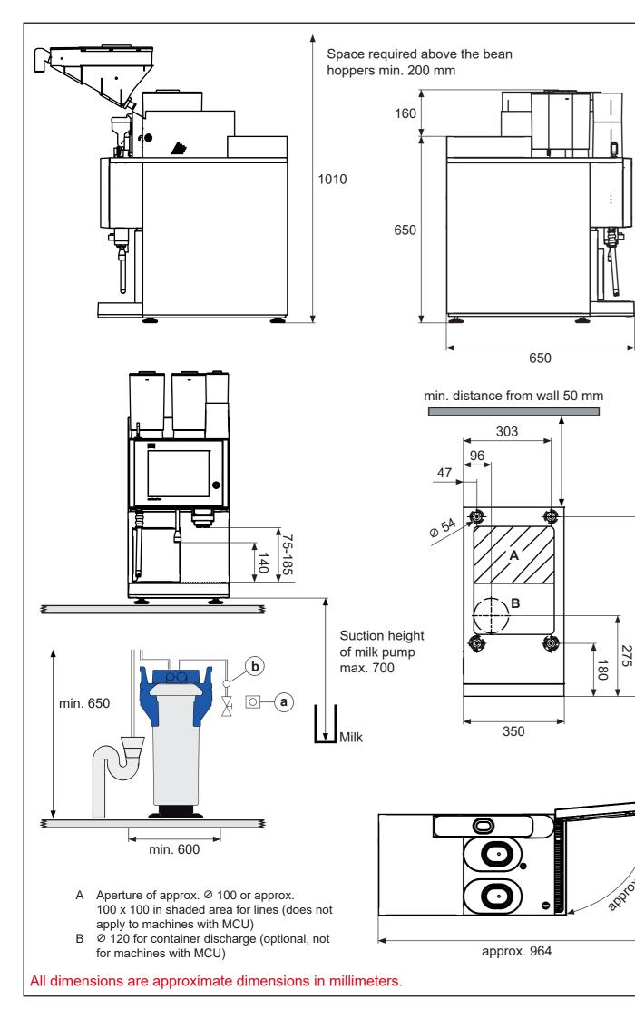
Dimensions (W x D x H): 350 x 650 x 810 mm I) Installation weight: approx. 70 kg Coffee bean supply:  $2 \times 3 | / 2 \times approx.$ 1000 g Instant container capacity: 1 x 1 l / 1 x approx. 1000 g Grounds drawer capacity: for approx. 40 portions
